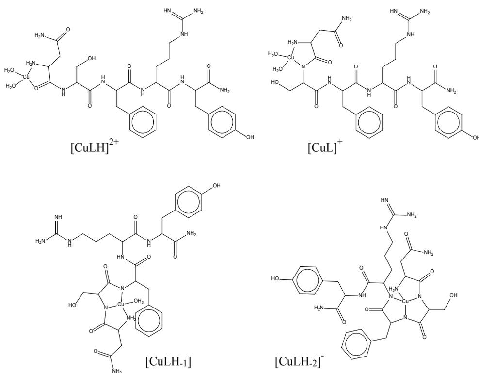
**Figure 1** Tetracoordinated Cu(II) complexes with NSFry-NH<sub>2</sub> in its protonated and deprotonated forms
