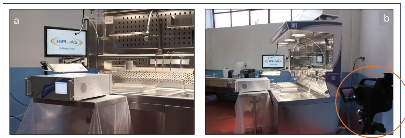
Figure 1 Test to assess formaldehyde gas containment on the worktop of the DFB900 grossing station: a) pre-calibrated laser infrared spectrometer; b) optical gas detection thermal camera
