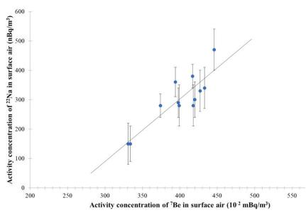
Figure 5 Correlation between yearly means of 7Be and 22Na concentrations in aerosols, averaged over the sampling locations
