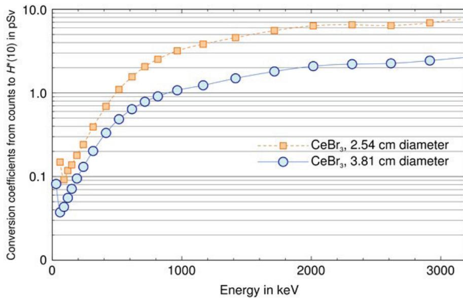
**Figure 1** Comparison of the energy-dependent conversion functions of two  $\text{CeBr}_3$  detector systems comprising of a 2.54 cm x 2.54 cm and a 3.81 cm x 3.81 cm scintillation crystal, respectively, based on simulated spectra calculated with the MC code GEANT 4, including the low-energy Library of EM-Livermore
