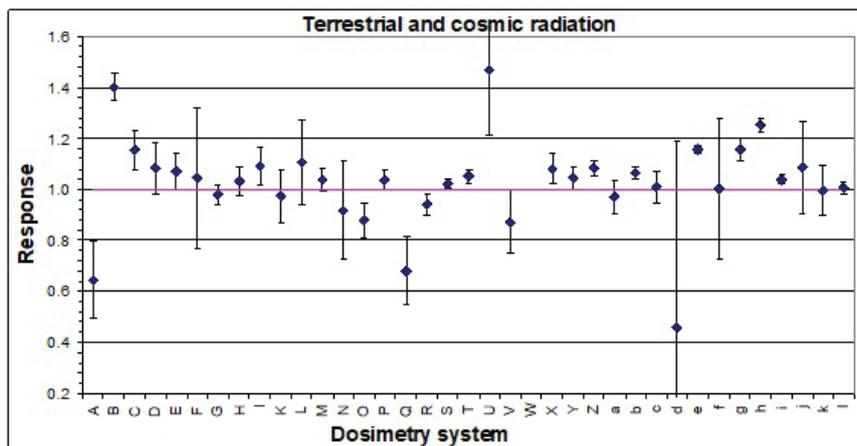
**Figure 4** Response of European dosimetry systems to combined terrestrial and cosmic radiation. The ideal response is exactly 1. The dosimeters were exposed for 6 months on the PTB reference measuring site for environmental radiation as shown in Figure 3. The systems (participants) are anonymised. Most systems are based on TLD detectors
